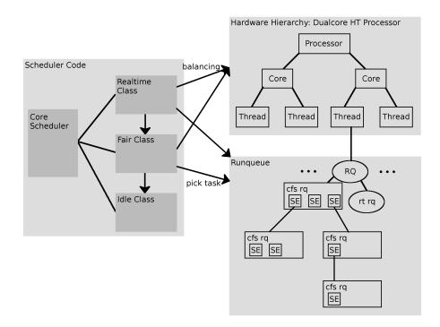
Figure 1: Diagram of the scheduling architecture in the Linux kernel. SE = Schedulable Entity, RQ = Runqueue, RT = Realtime, CFS = Completely Fair Scheduler, HT = Hyper Threading
