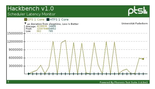
Figure 6: Latency at hackbench with 300 processes
