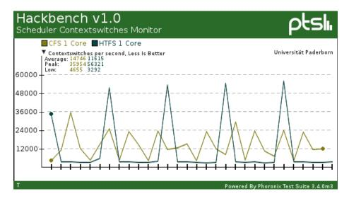
Figure 4: Context switches at hackbench with 300 processes.
