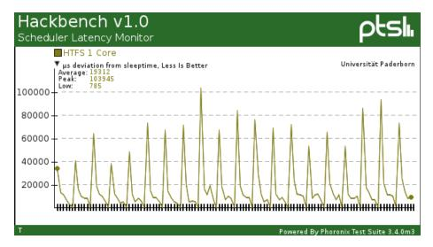
Figure 5: HTFS latency at hackbench with 300 processes
