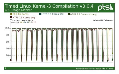
Figure 26: Kernel Compilation CPU usage.
