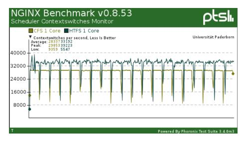
Figure 13: Context switches per second for NGINX Benchmark.
