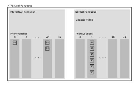
Figure 2: An overview over the HTFS specific runqueue structure named Dual Runqueue
