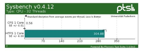
Figure 8: Deviation from the average work done per thread.
